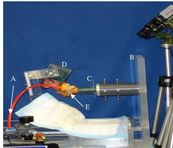
Figure 1. Experimental setup including: A) Air supply B) custom shoulder jig C) humerus D) scapula and E) capsule.
